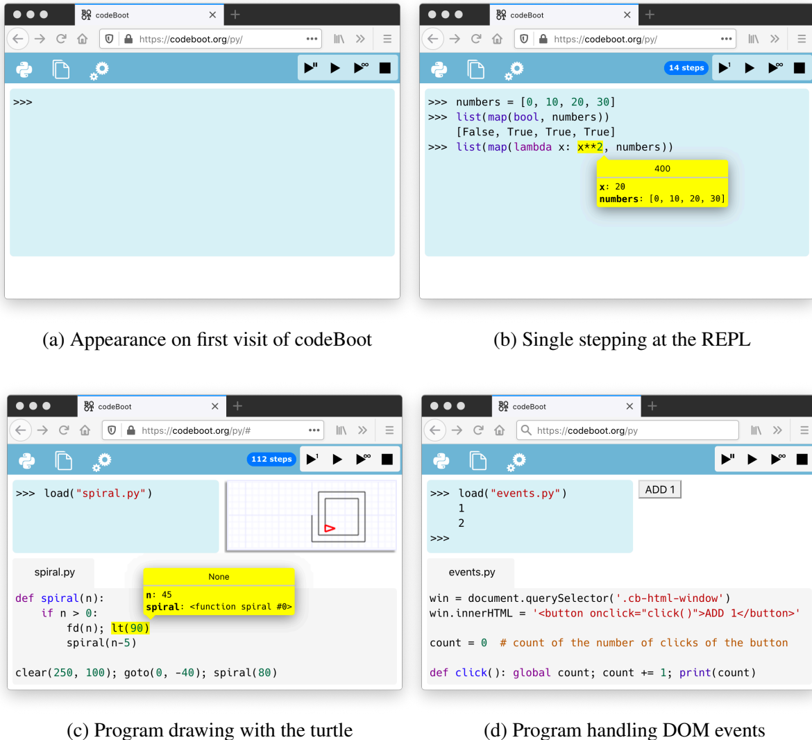
Figure 1: The codeBoot user interface and its features (each screenshot is a clickable hyperlink)
